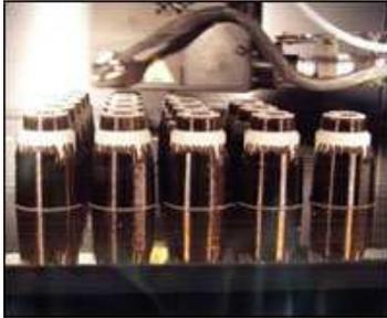
With direct-digital manufacturing, the TDF can produce batches of components with the FDM process.
