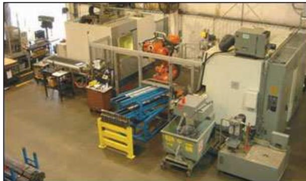
At Smith's Machine, DMG Twin machines with Siemens Sinumerik 840D CNCs are fed by the robot that loads and unloads the turning center and the four-axis milling machine, and rotates the parts through a queuing station before engraving and placing the part on the engraver.
