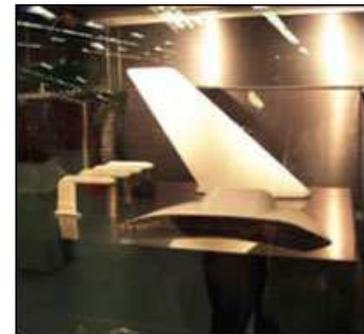
Antenna and other components are manufactured by a Fortus FDM machine.
