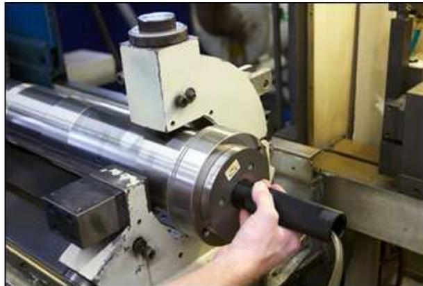
HSK 125 spindle shaft ID taper check. Photo courtesy AME's Bill Edmundson
