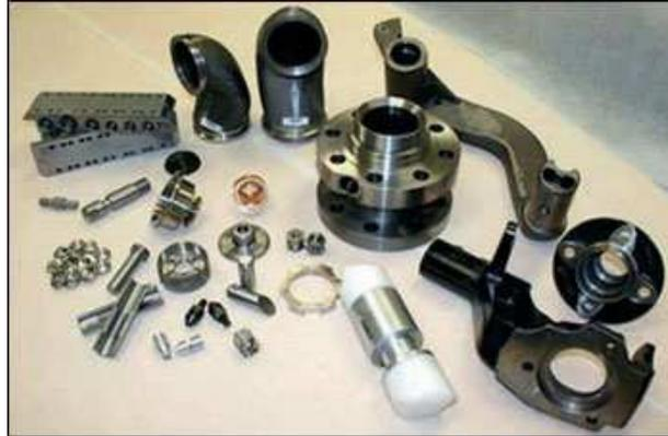
Representative automotive parts produced at Smith's Machine include a tow bushing, valve block, spare tire arm, stainless spinnerette, steering knuckle, propane valve, and several marine diesel turbocharger parts supplied to the Mercedes facility in Tuscaloosa County and other OEMs.
